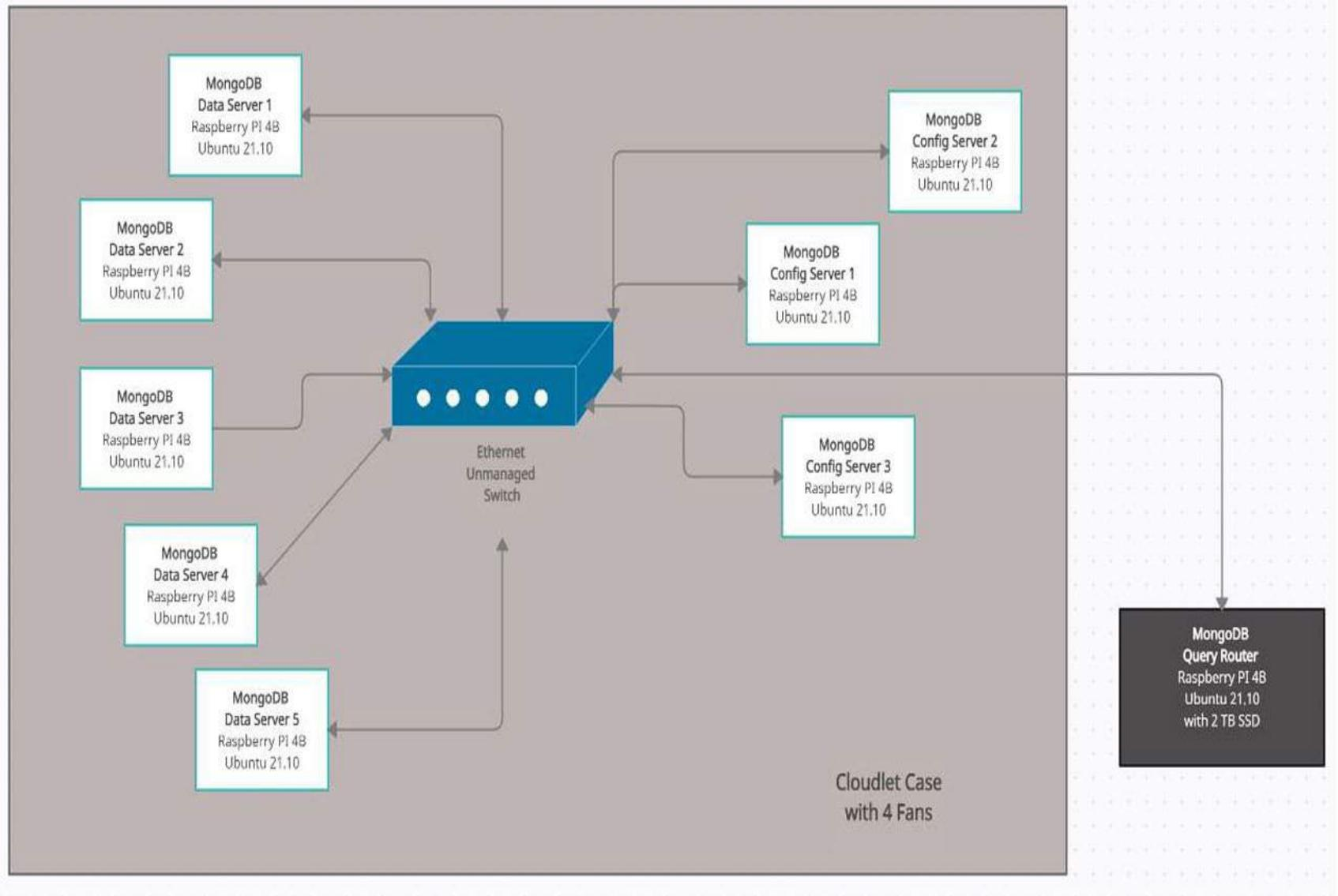
**Figure 1: Rpi Model 4B Cluster Architecture**
